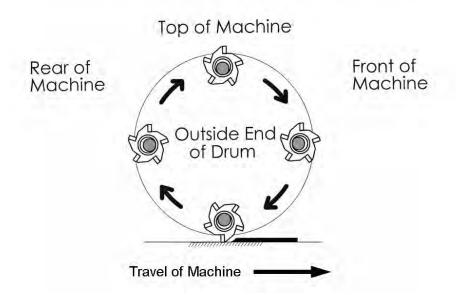
Correct rotation of the Milling Cutters is critical to successful resurfacing and to insure maximum wear life. Drum and cutter assembly should be mounted so that cutters are rotating towards the front of the machine as indicated above.
